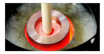
The optimal thermal coupling from the block to the test item is achieved by an exactly fitted adapter sleeve. These adapter sleeves can be produced according to customer specifications, enabling the simultaneous calibration of different temperature sensors.
